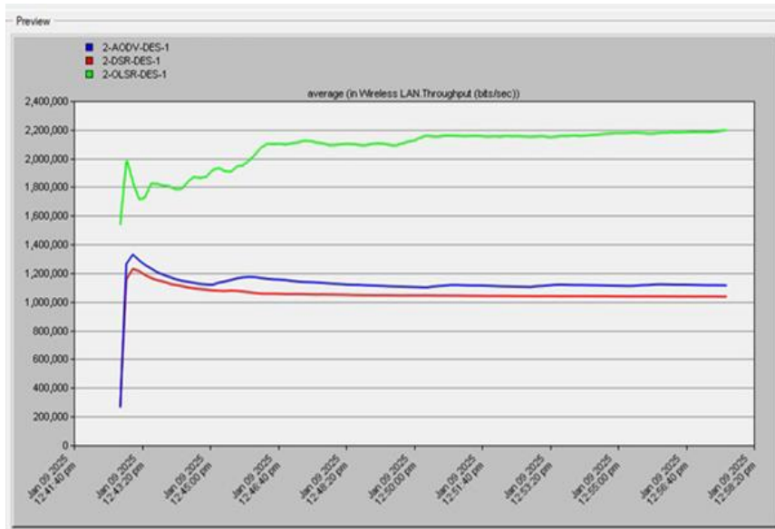
Figure 8. Average Throughput in a Medium-Scale MANET
